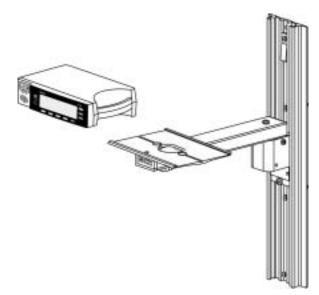
Figure 4: GCX Poly-mount (vertical wall mount with 19-inch channel)
