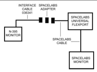
Figure 21: SpaceLabs Connection
