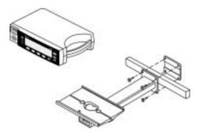
Figure 5: GCX Poly-mount (horizontal wall mount with rail adapter)
